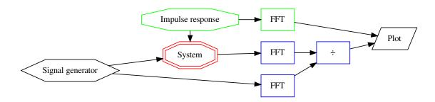
Adding the measured transfer function is done through connections, just like the other connections, that have been established before. It is noteworthy though, how the spectrum of the impulse response is added by simply calling the respective methods and without relying on the functionality of the *Connectors* package. This shows, that the decorated methods can still be used as normal methods, even when they are extended with the functionality of a connector.
