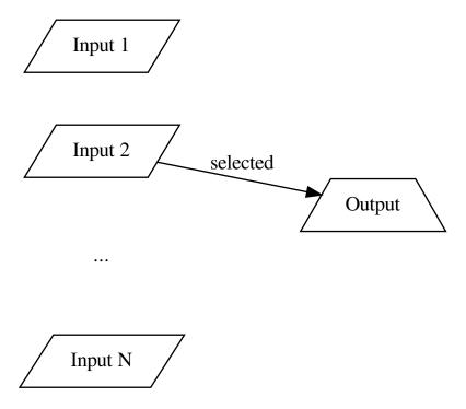
A very common application for multiplexers is signal routing in electronic circuits, for which there is a huge variety of integrated circuits, such as the 74LS151 or the CMOS 4097. In some occasions, a multiplexer can also be helpful to implement a processing networs, which is why the Connectors package provides the Multiplexer class.
